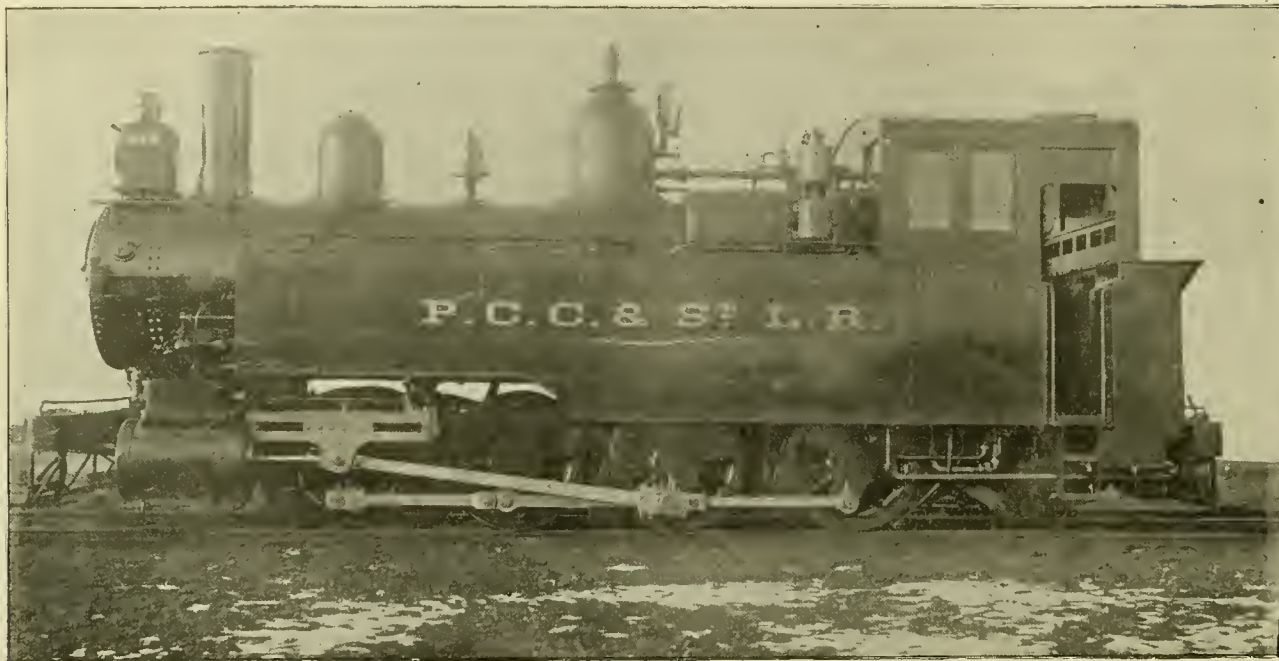
Locomotive for a Six Per Cent. Grade.—Pittsburgh, Cincinnati, Chicago & St. Louis Railway.
